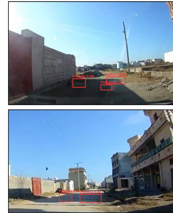
Fig. 6. Real-world evaluation of the YOLOv11n model for pothole detection. The model successfully detects potholes even in the presence of shadows, demonstrating its robustness to challenging lighting conditions.
